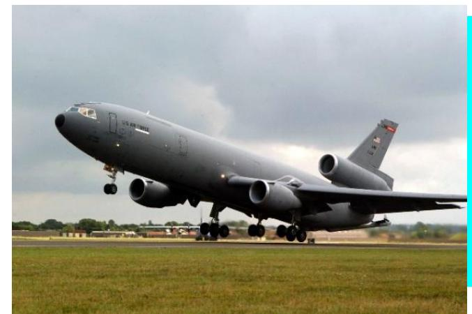
10s, the tanker/transport is 181 feet 7 inches long, has a wingspan of 165 feet 4 inches and a tail height of 58 feet 1 inch. Gross takeoff weight of the KC-10A is 590,000 pounds (267,619 kg), up from 555,000 pounds for the standard intercontinental commercial model.
